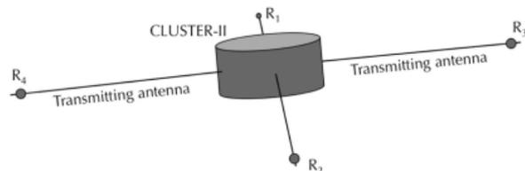
The WHISPER instruments makes both passive recordings and active soundings in the 2–80 kHz band; data is presented as a **E** field spectrogram.
