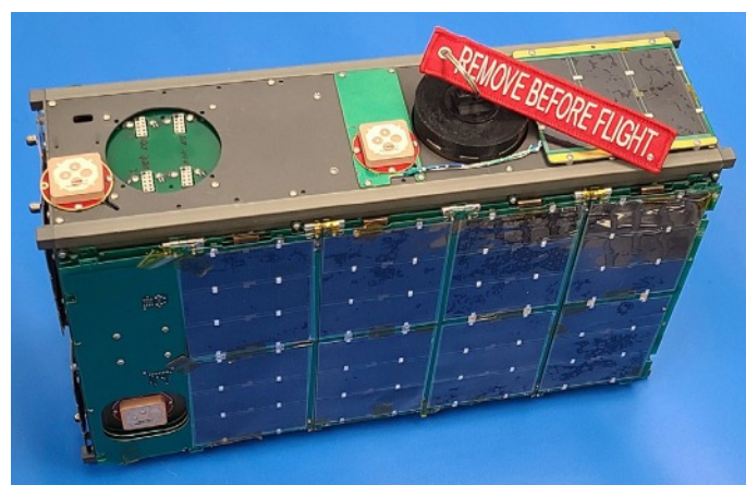
Fig. 2: DUPLEX satellite with deployable solar panels in stowed configuration
