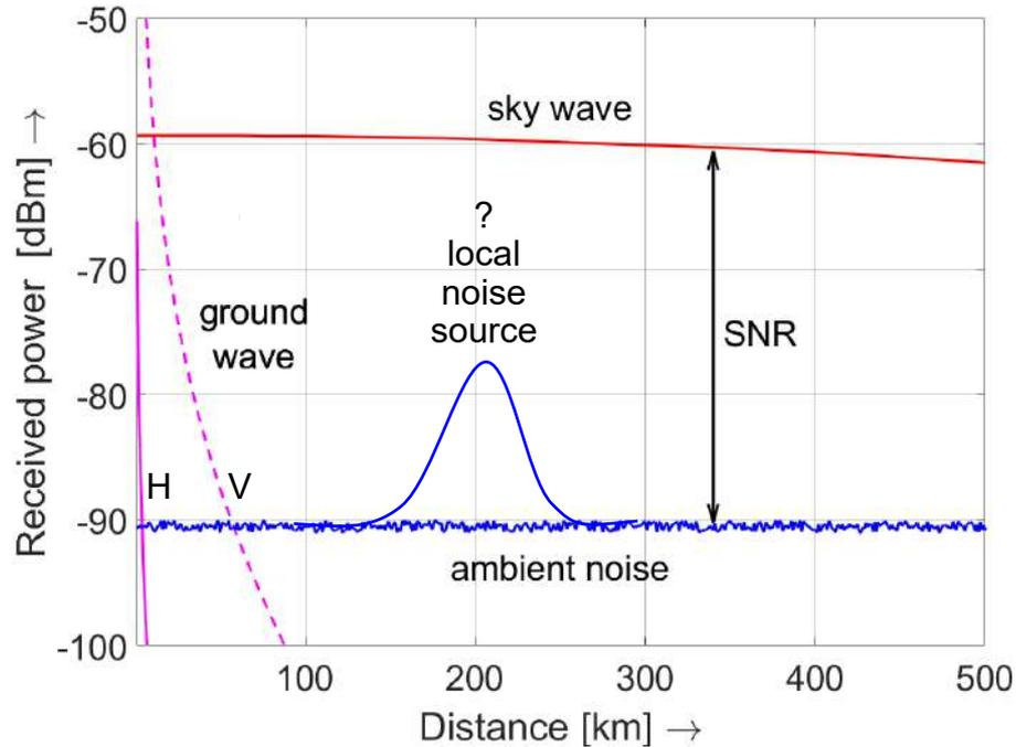
Simulated signal strength assuming isotropic antennas:
