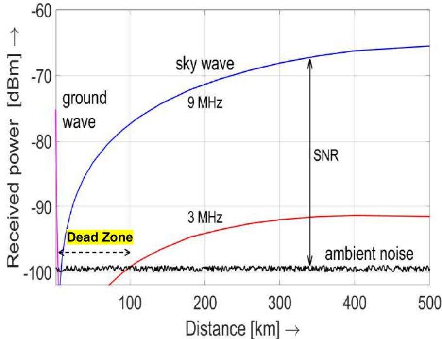
Simulated signal strength using real antennas
