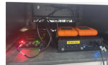
**GNSS scintillation receiver**
